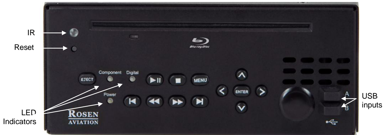
Figure 1 Rosen Blu-ray DVD Player front case showing LEDs and control buttons
