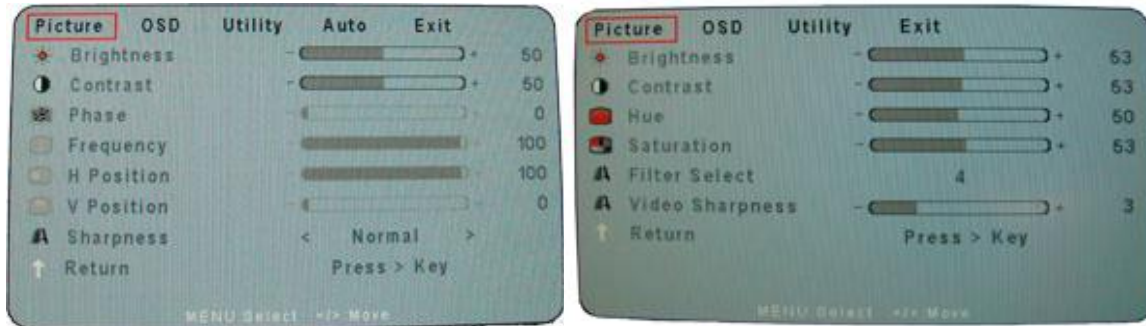
Figure 3 Main Menu for analog RGB mode (left) and for composite mode (right)
