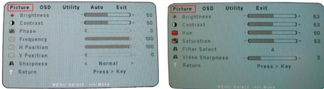
Figure 26 Main Menu for analog and digital RGB modes (left) and for composite mode (right)
