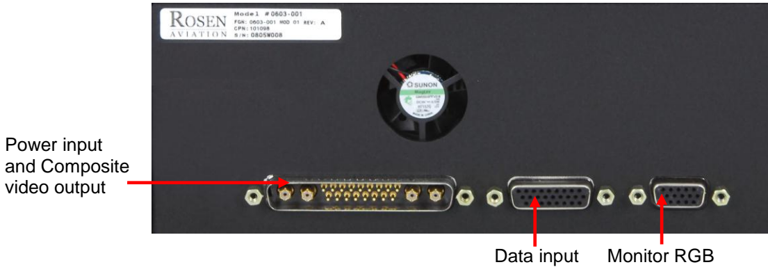
Figure 2 RosenView LX rear panel connections
