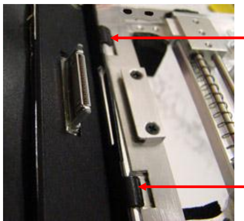
Figure 8 Proper alignment of housing and bezel mounting tabs
